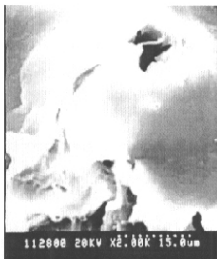
图 3-1 (c) SF/PP 复合材料无缺口冲击破坏断口的 SEM 照片 ( W_{pp}=60\% , SF=5mm ) Fig3-1(c) SEM photomicrograph of non-notched impact fracture surface of short sisal fiber/PP composites ( W_{pp}=60\% , SF=5mm )
